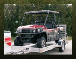
No worries finding the right location to hook a securement strap. There are three securement locations at the front and every 12" on the sides. All units have a 16" deck height. The ramp is 48" long.
